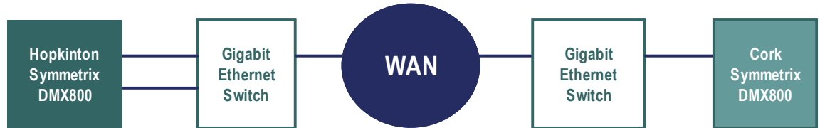
Figure 2: EMC SRDF/A Connection Topology (Simplified)
