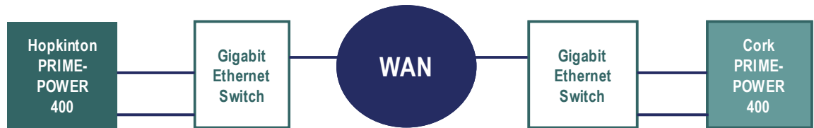
Figure 1: PRIMEPOWER 400 Connection Topology (Simplified)
