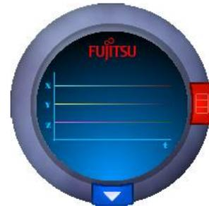
Inside select Fujitsu mobile PCs there is an accelerometer that constantly senses for any sudden movement, including free falls, excessive vibration, or sudden impacts. Fujitsu Shock Sensor monitors movement from three axes: front-to-back, side-to-side, and up-and-down. The sensitivity of the Shock Sensor can be adjusted by the user to accommodate different working environments.
