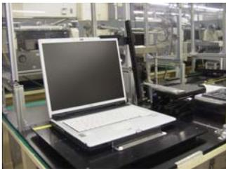
After several thousand test cycles, the display must work normally at any angle.
