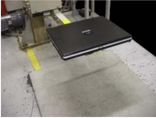
After a number of free-fall tests from different heights at various angles, the unit and all programs must function normally. No damage or cracking is allowed in any part of the test sample. There should also be no damage and no ejection of media cards or cables.
