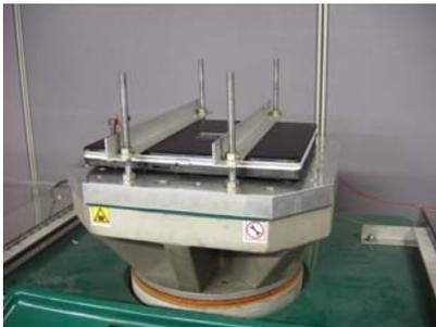
Reliability in data protection for the hard disk drive, and durability of the LCD and optical disc drive is evaluated under accelerated severe conditions. This test contains operating and non-operating vibration tests, shock tests, and operating and non-operating drop tests.
